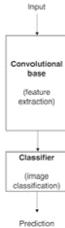
Figure 3.20: Typical CNN architecture
